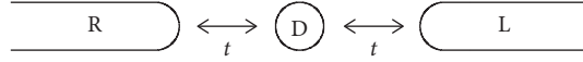
FIGURE 1: Schematic diagram of a superconductor/quantum dot/superconductor (S/QD/S) junction. t denotes the tunneling amplitude between the leads and the QD.
