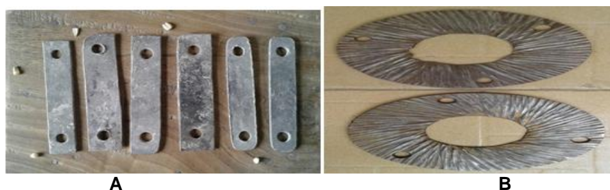
Fig. 3. Grinding Machine Discs: (A) Hammer plates; (B) Disc plates
