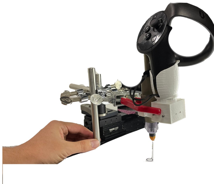
Fig 7. Subject performing the 2-D printed circle experiment. The figure shows one subject conducting the experiment with manual movement of the linear stage. A 10 mm circle is printed on a sheet of paper. The subject traced the circle by using the linear stage manually.
