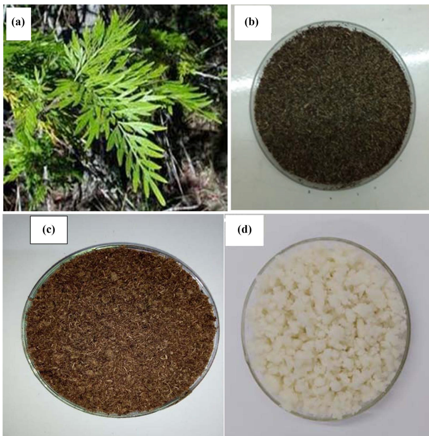
Figure 1. Images of (a) fall leaves, (b) raw sample, (c) unbleached cellulose, and (d) bleached cellulose.
