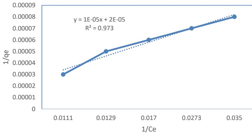
**Fig. 3. Langmuir isotherm plot for the adsorption of congo red**
