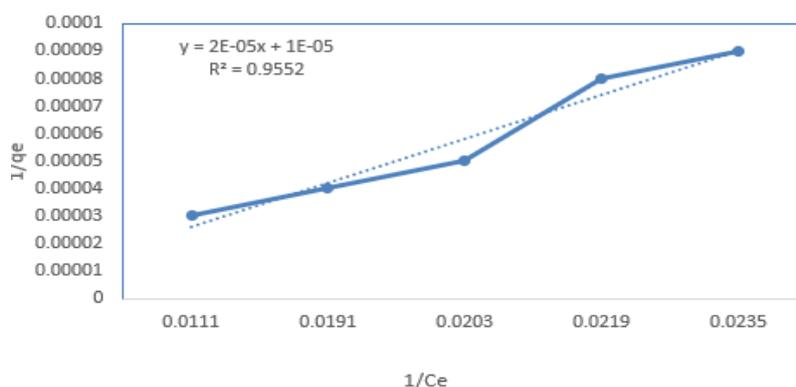
**Fig. 1. Langmuir isotherm plot for the adsorption of Methyl red**
