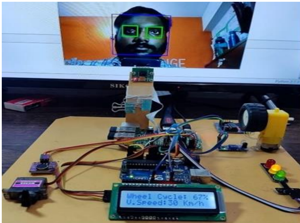
Fig. 9. The face and eyes of the driver are detected, the Yellow LED and Green LED are on, the Red LED is off. The wheel motor is rotating, and the servo motor is at 90°
