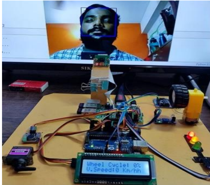
Fig. 10. The face of the driver is detected but the eyes are not detected. The Yellow and Red LEDs are on, and the Green LED is off. The wheel motor is not rotating, and the servo motor is at 180°
