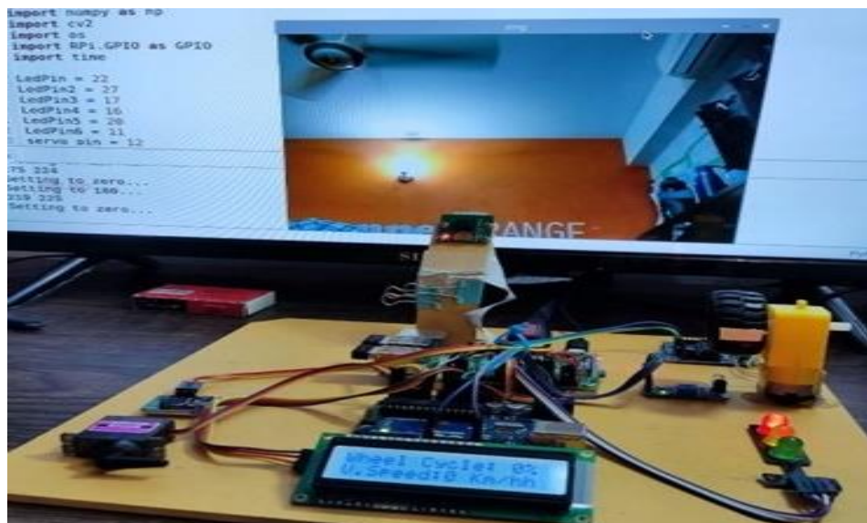
Fig. 11. The face and eyes are not detected, the Red LED is on, Yellow and Green LEDs are off. The wheel motor is not rotating, and the servo motor is at 180°
