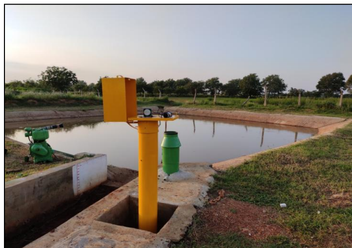
Plate 2a. Image showing setup of Thalimede data encoder, data logger and self recording rain gauge at the inlet section of form pond
