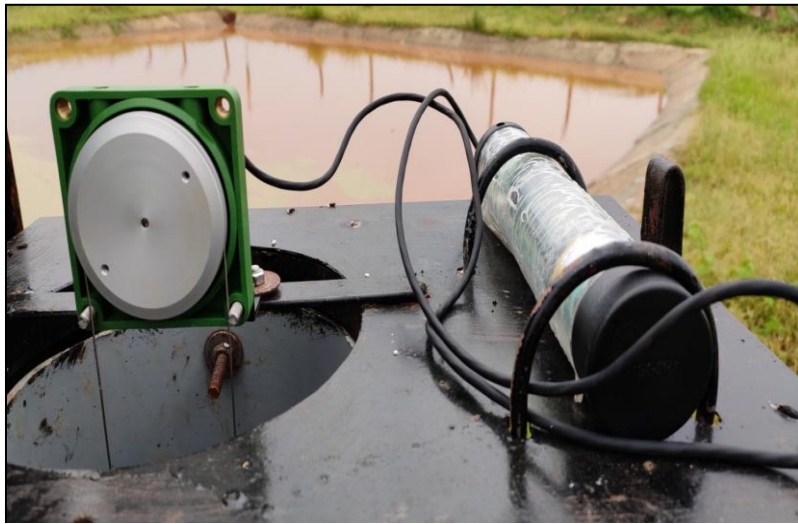
Plate 2b. Close view of thalimede data encoder and data logger used in the study area
