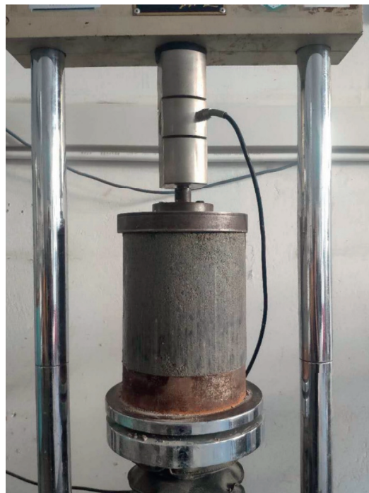
FIGURE 3: Pavement material strength tester.
