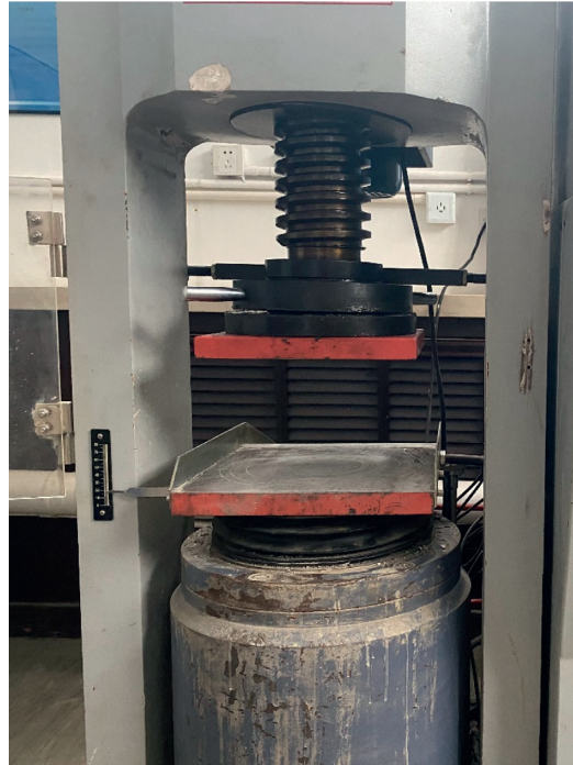
FIGURE 2: 2000 kN press machine.
