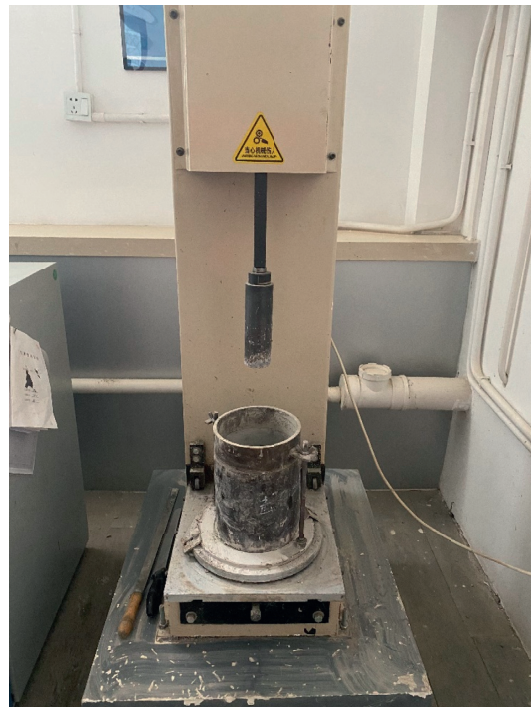
FIGURE 1: Compaction test apparatus.
