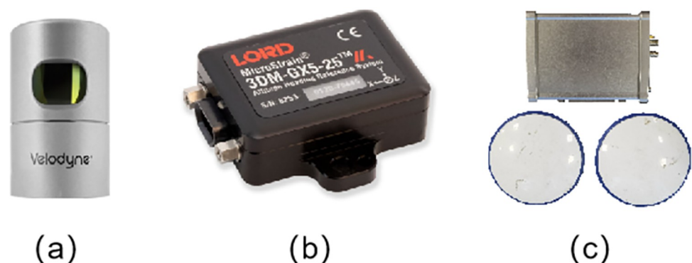
Fig 6. The sensor setup used in our experiments: (a) a Velodyne HDL-32E surround LiDAR sensor, (b) a 3DM-GX5 IMU, and (c) a Trimble BD982 GNSS receiver module with antennas.
