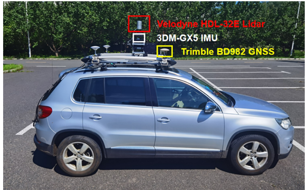
Fig 7. Recording platform (Volkswagen Tiguan) with sensors.
