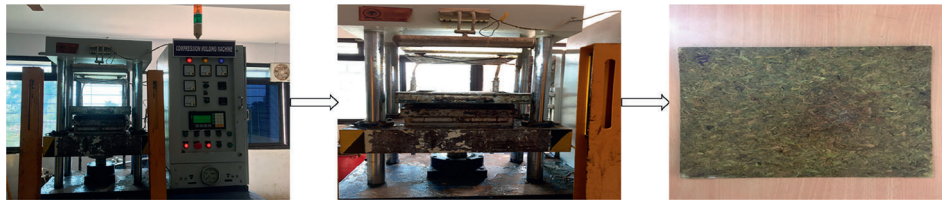
FIGURE 2: Fabrication process of water hyacinth plant fibre composite.
