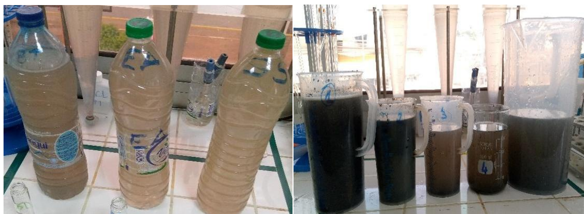
Fig. 1. Samples of wastewater (A) taken at the entrance to the WWTP in the buffer basin (BT), the anaerobic effluent channel (EA) and at the WWTP outlet (SS) and anaerobic sludge from the UASB reactor (B)
