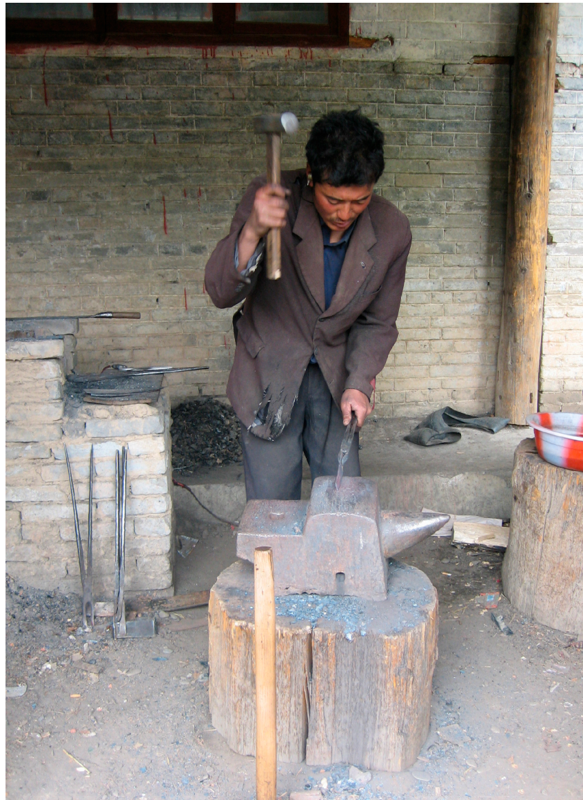
Figure 12. The Zhang ngu khog blacksmith at work at the single anvil located close to the hearth. A bowl on the right atop a wooden stump holds water and clay for iron quenching.
