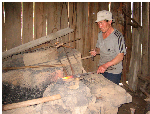
Figure 4. The Lha yul blacksmith heats iron on the coals at the stone hearth with his left hand and operates the box bellows with his right one, delivering a constant supply of oxygen to the coals and raising the combustion rate and temperature output. He made both the hearth and the bellows himself.
