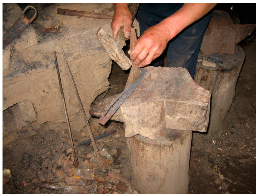
Figure 5. The Lha yul blacksmith uses a chisel and hammer to cut a hot metal piece lengthwise to form a repair piece for a loom.
