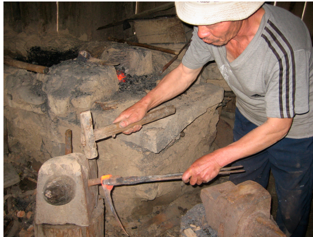
Figure 3. The blacksmith uses a piercing tool mounted on an anvil to help work the hot iron. This work takes place very close to the hearth.
