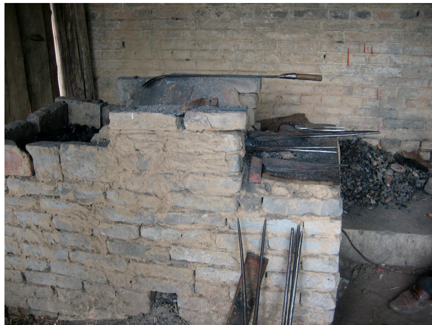
Figure 11. The hearth in the Zhang ngu khog workshop has a shelf (right side) for setting aside small tools that are frequently used by the blacksmith; the opening at the bottom center of the hearth is used for removing burnt coal ashes and clinker. A pile of these can be seen behind the hearth, awaiting disposal.
