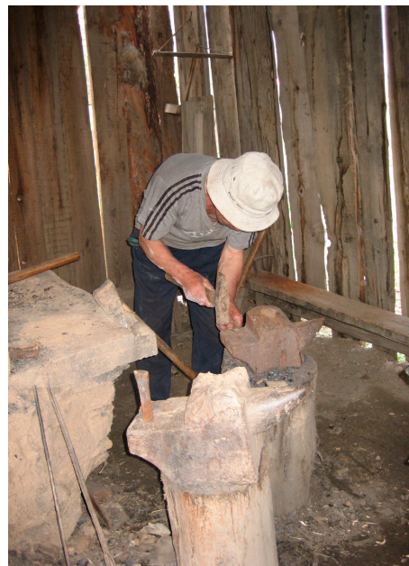
Figure 2. The Lha yul blacksmithing shed. Two anvils are located very close to the hearth. The blacksmith is using a forging hammer.
