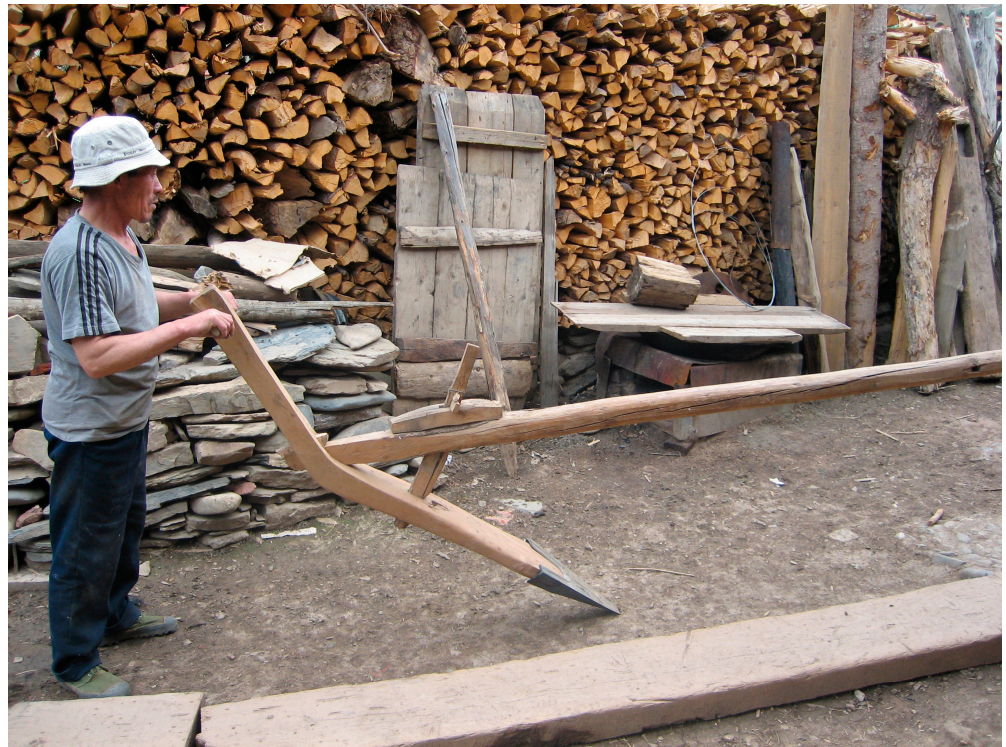
Figure 9. The Lha yul blacksmith forged an iron plow bit and attached it to a complex wooden plow that he constructed in his courtyard.
