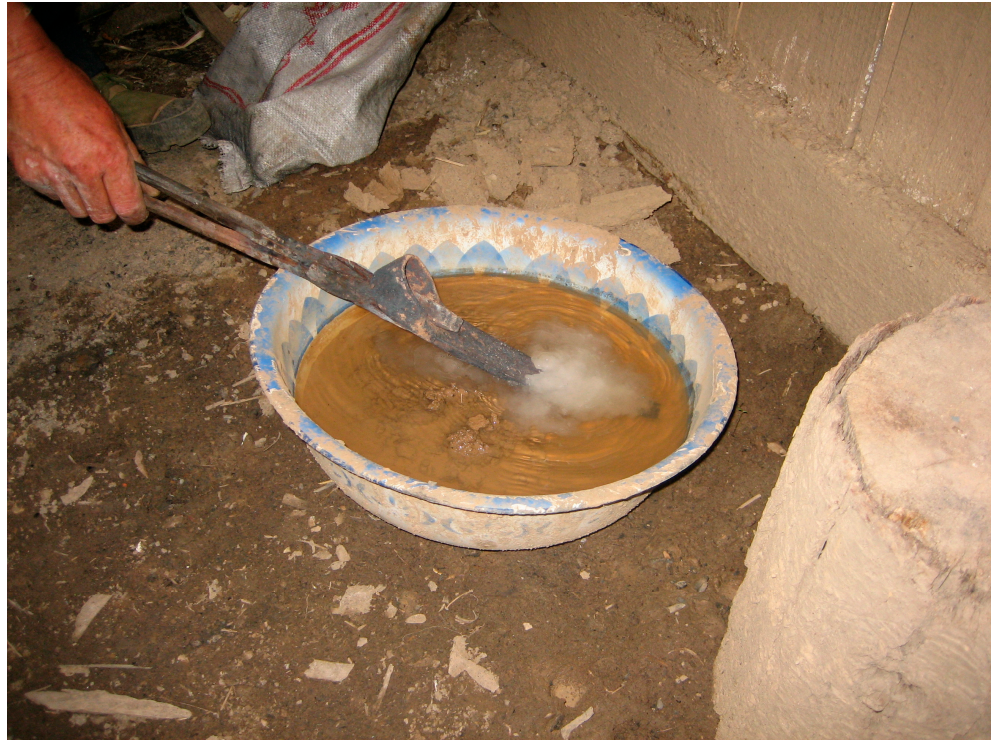
Figure 7. The Lha yul blacksmith quenches a finished piece of forged iron, rapidly cooling it in a bowl of water mixed with fine clay.
