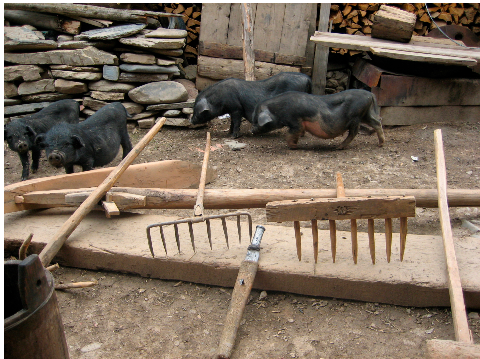
Figure 8. Some of the tools the Lha yul blacksmith makes, repairs, and assembles in his courtyard include a rake with iron tines, a rake with wooden tines attached to the head with iron rivets, and a sheathed knife used for cutting roof tiles.
