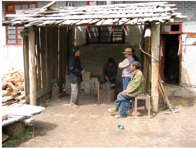
Figure 10. The Zhang ngu khog blacksmithing workshop serves as a social center in this village. The blacksmith is working on his sole anvil next to a brick hearth. The back wall of the workshop is an outer wall of the blacksmith's home. The front is open and facing the courtyard.
