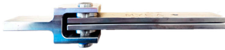
Figure 2. Bearing metallic jig for type-A bearing test of a double-shear joint.
