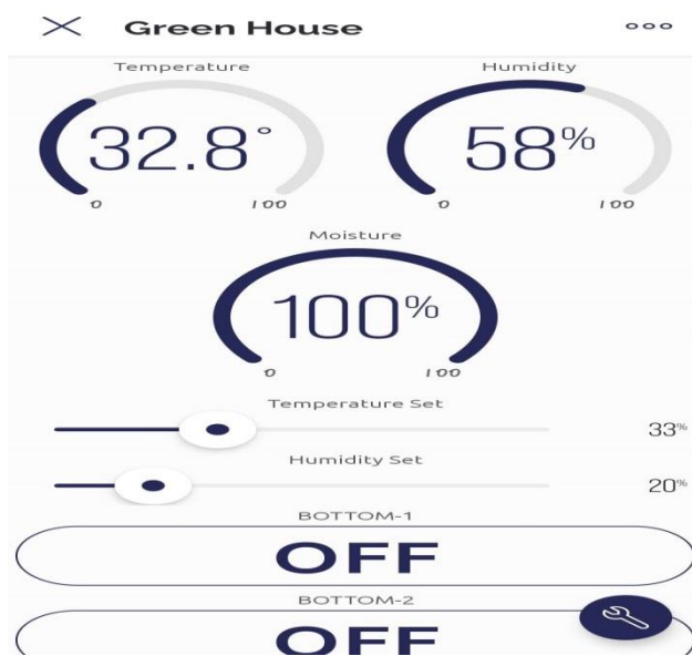
Fig. 10. Monitor moisture Sensor data via Blynk IoT app
