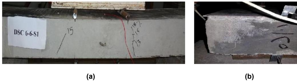
Fig. 12. View after failure load of the specimen DSC 6-6-S1 with wide crack in concrete (a), and close up view of the right side corner showing longitudinal cracks in concrete (b)
