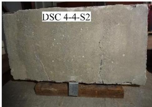
(b) Splitting cracks in concrete core
