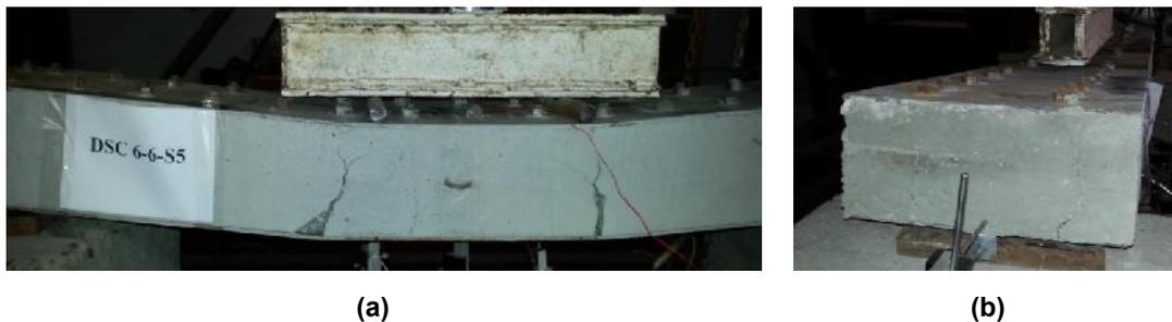
Fig. 16. View after failure load of the specimen DSC 6-6-S5 with wide crack in concrete (a), and close up view of the right side corner showing longitudinal cracks in concrete (b)
