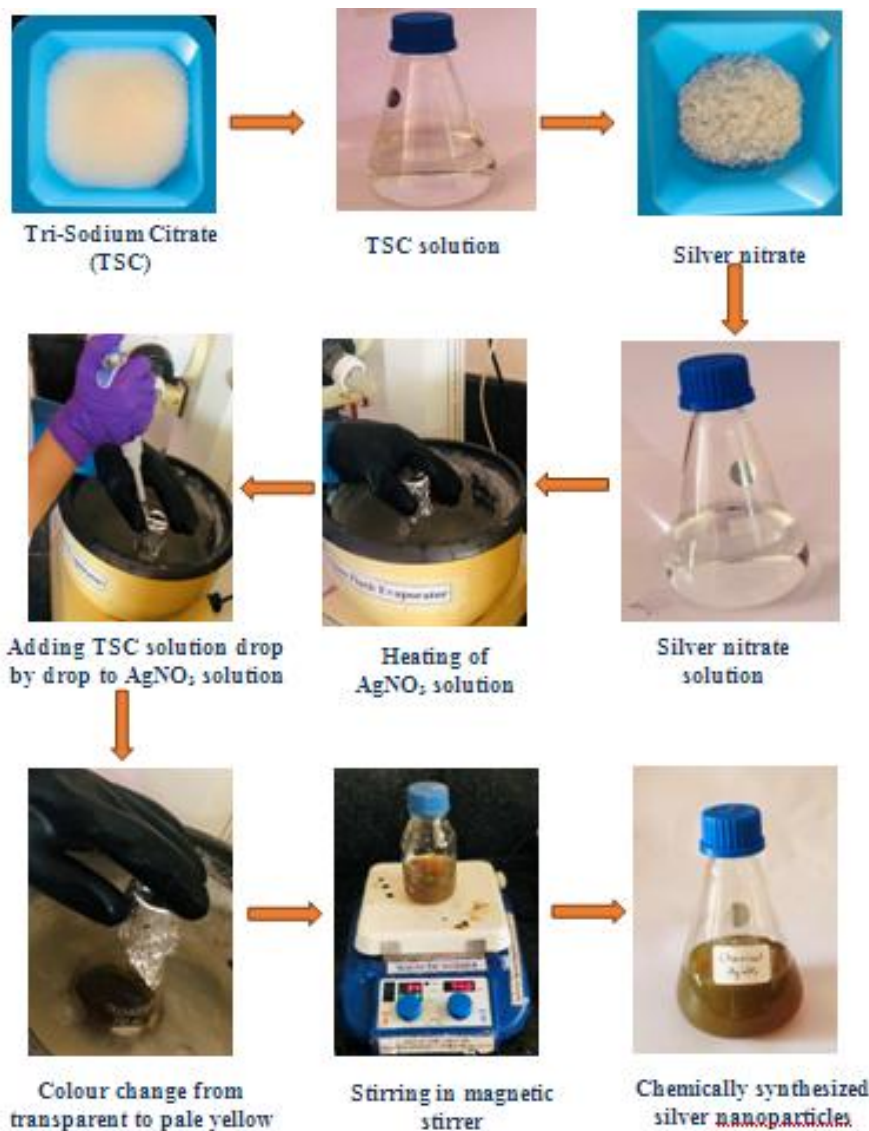
Fig. 2. Process flow chart for chemical synthesis of Ag NPs using TSC
