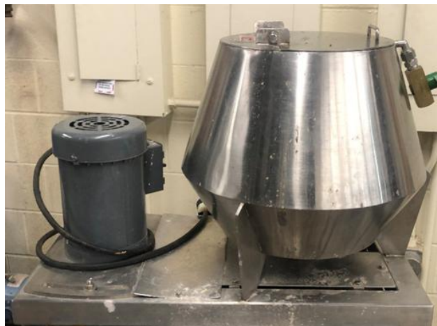
Fig. 4. Low consistency laboratory repulper [35]
