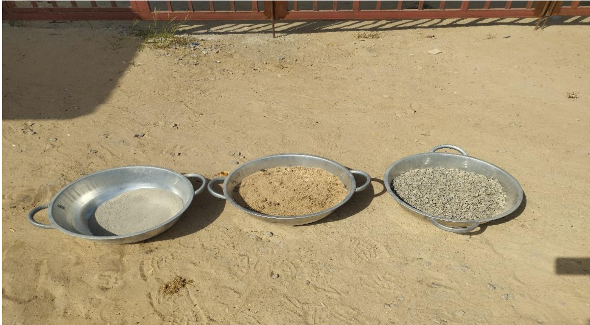
Plate 1. Constituent materials: from left to right: Portland cement, Sand, Granite
