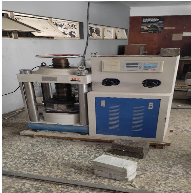
Plate 5. Crushing of control and sample paving stones
