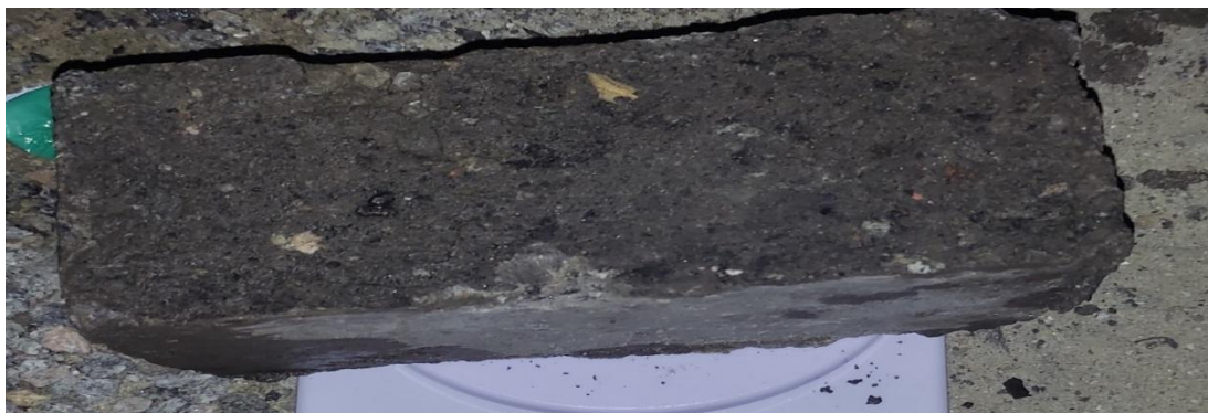
Plate 4. Sample 1, (waste plastic bound paving stone)
