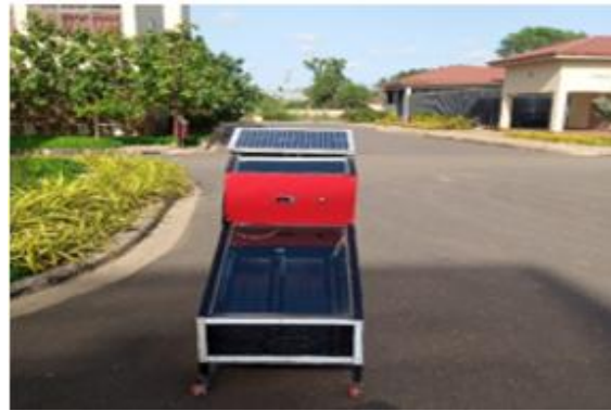
Fig. 4b. Constructed solar dryer
