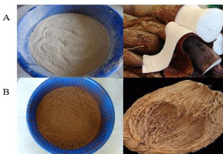
Fig. 2. Agricultural waste materials for super absorbent polymer production. A: Cassava mesocarp powder obtained from cassava mesocarp B: Coconut coir dust obtained from coconut husk
