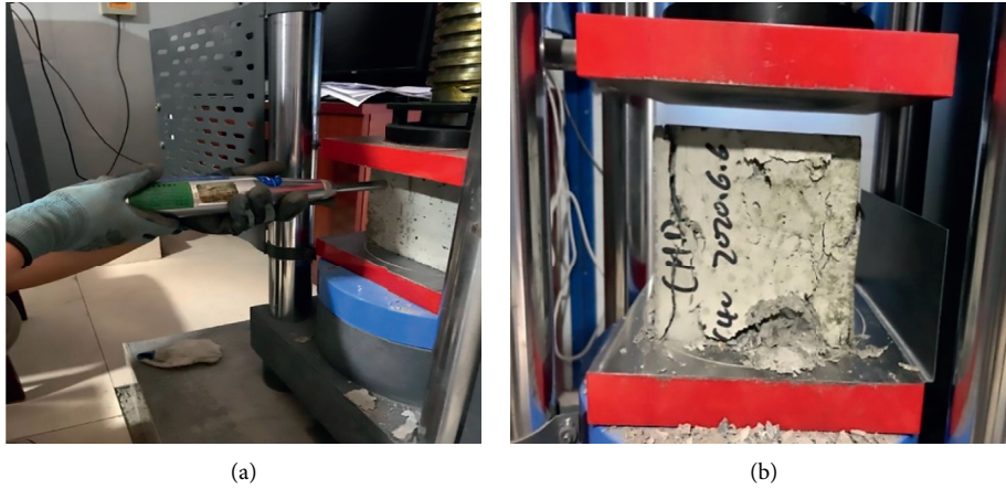
FIGURE 1: The rebound hammer test and compressive strength test of concrete specimens: (a) rebound hammer test and (b) destructive compressive strength test.
