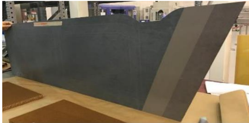
Figure 4. Demonstrator trailing edge panel of a horizontal tail, an example for the combination of conventional materials like carbon fibers with partly bio-based epoxy resin developed during the ECO-COMPASS project.
